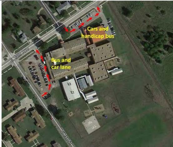
The bus and car lane on the west side can only allow 14 vehicles to stack off of the right-of-way. The car and handicap lane on the north side only allow for 12 vehicles to stack off of the right-of-way. Current layout of the parking/drives is outdated for the student/teacher population. Several areas between parking and the buildings require students and teachers to cross bus and parent traffic with no designated walkways.
